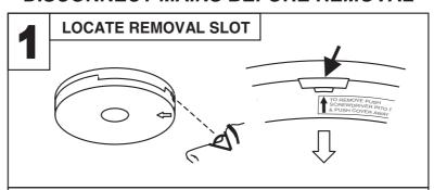
LOCATE THE ARROW ON THE FRONT FACE OF THE ALARM. THE SLOT IS LOCATED DIRECTLY ABOVE THE ARROW.
